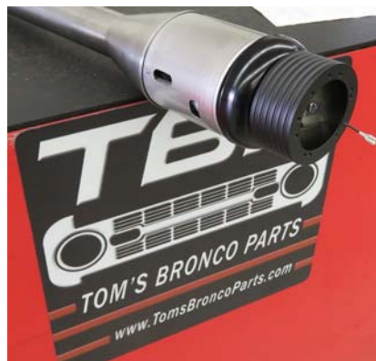
Fig 5. - Install wheel hub, lining up the three 1/4" holes with the adapter hub. Be sure elongated hole is lined up, allowing the horn wire to pass through. It will Only line up one way. The horn pedestal from the tilt column fits through this hole.
