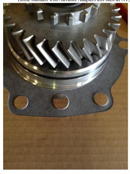
Notice how the hole in the gasket is NOT large enough to fit the bearing retainer.
