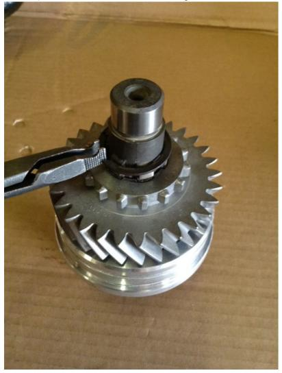
Install the snap ring into the groove on the coupler shaft.
