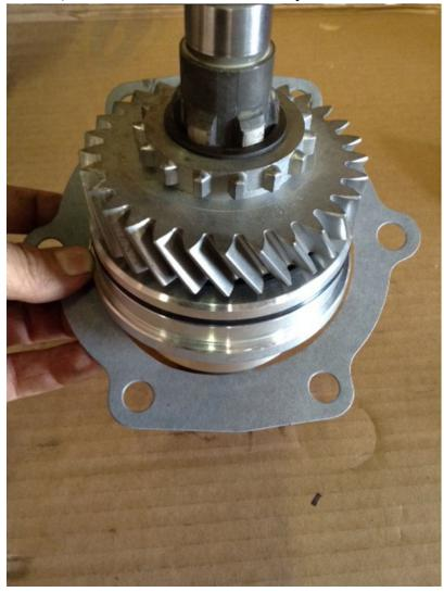
After trimming, the gasket should be able to slide over the bearing retainer.
