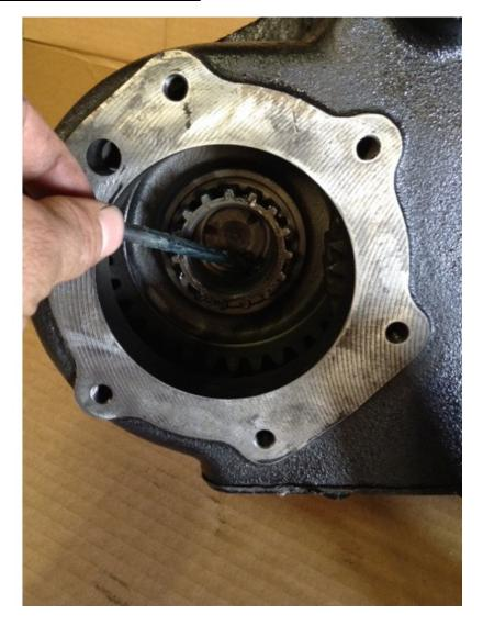
Apply grease to cup portion of rear output shaft. This is to hold the pocket bearings while installing them.
