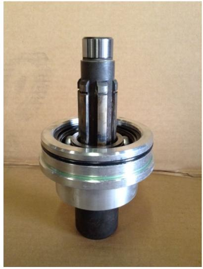
Slide the bearing and retainer over the coupler shaft. Note how the bearing retainer is oriented to the shaft. Drive the inner race of the bearing down along the shaft until seated on the coupler shaft.
