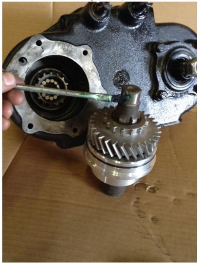
Apply a thin film of grease to the adapter shaft where the pocket bearings will ride.
