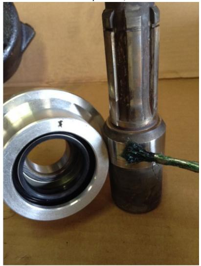
Apply a thin film of grease to the seal surface area of the coupler shaft. Also apply grease to the inside surface of the seal within the adapter bearing.
