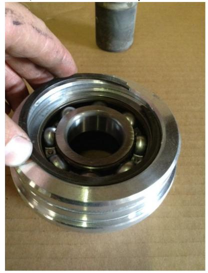
Install the snap ring to hold the bearing from working its way out
