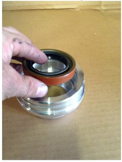
Install new Adapter Seal into Bearing Retainer. We STRONGLY recommend a NEW adapter seal when replacing the transfer case.
