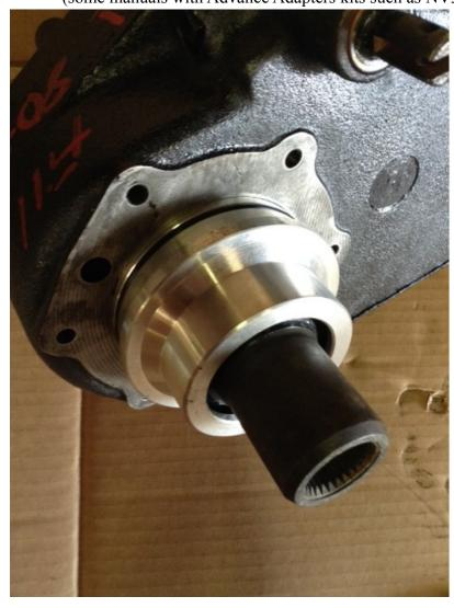
Install the bearing retainer assembly into the transfer case housing. Lightly tap on the bearing retainer to seat it with a dead blow hammer. DO NOT hit the shaft!
