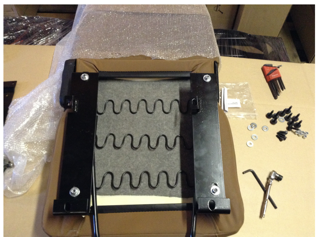
Illustration 2: Driver Seat Bracket Installed
