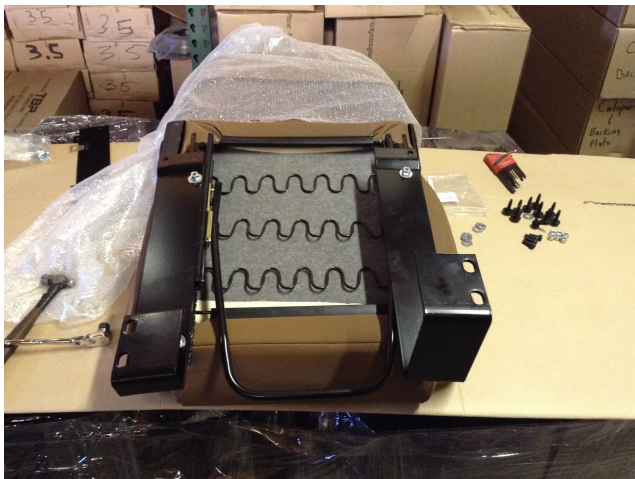
Illustration 1: Passenger Seat Bracket Installed
